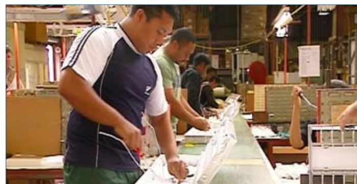
Assembling light fittings.
